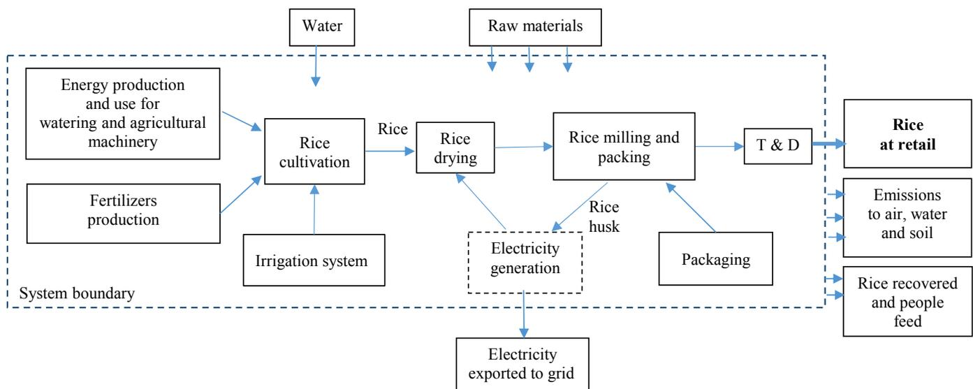
**Fig. 1.** System boundaries adopted in this study (T & D = transport and distribution). The dashed line indicates stages considered only in the new system.
