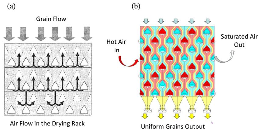
Fig. 8. Drying systems: (a) conventional drying rack, (b) new system of drying rack.
