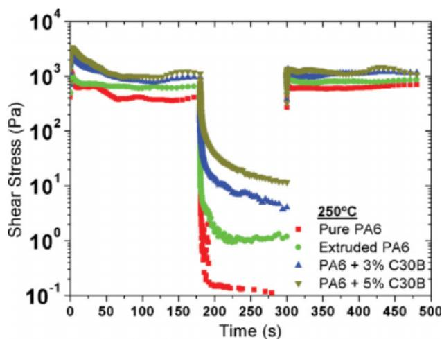
**Figure 9** Stress growth and stress relaxation experiments of the extruded nanocomposites, at 250°C and  $\dot{\gamma}_0 = 1.0 \text{ s}^{-1}$ . [Color figure can be viewed in the online issue, which is available at [www.interscience.wiley.com](http://www.interscience.wiley.com).]
