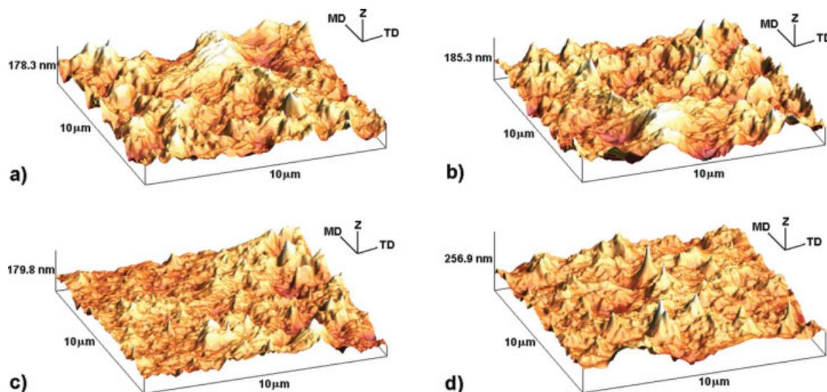
**Figure 13** AFM micrographs of the surface of the blown films of: (a) Pure PA6, (b) Extruded PA6, (c) PA6 + 3% C30B, and (d) PA6 + 5% C30B. [Color figure can be viewed in the online issue, which is available at [www.interscience.wiley.com](http://www.interscience.wiley.com).]
