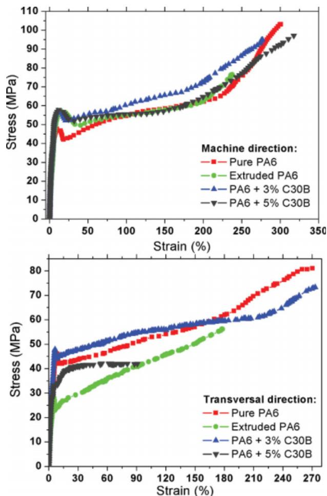
**Figure 11** Tensile curves of the blown films along MD and TD. [Color figure can be viewed in the online issue, which is available at [www.interscience.wiley.com](http://www.interscience.wiley.com).]
