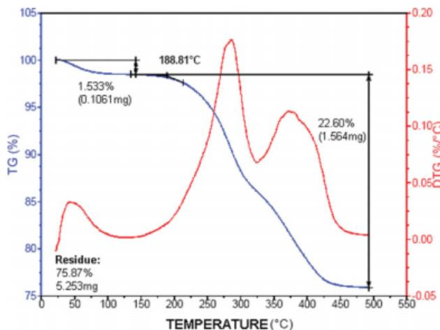
**Figure 3** Thermogravimetric analysis of the C30B nanoclay. [Color figure can be viewed in the online issue, which is available at [www.interscience.wiley.com](http://www.interscience.wiley.com).]
