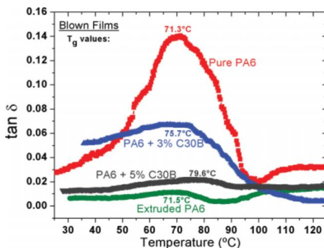
**Figure 12** DMTA analyses of the blown films. [Color figure can be viewed in the online issue, which is available at [www.interscience.wiley.com](http://www.interscience.wiley.com).]
