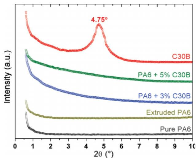
**Figure 4** WAXD diffractograms of the extruded nanocomposites. [Color figure can be viewed in the online issue, which is available at [www.interscience.wiley.com](http://www.interscience.wiley.com).]
