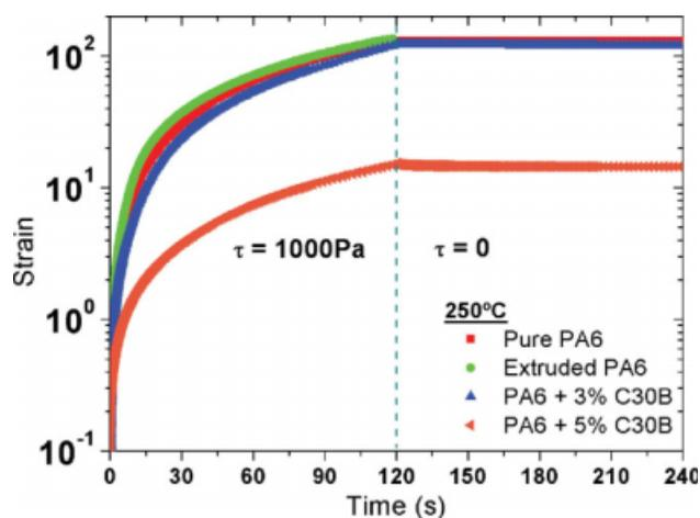
**Figure 10** Constrained recoil after cessation of steady state shear flow ( $\tau = 1000 \text{ Pa}$ ), at 250°C. [Color figure can be viewed in the online issue, which is available at [www.interscience.wiley.com](http://www.interscience.wiley.com).]
