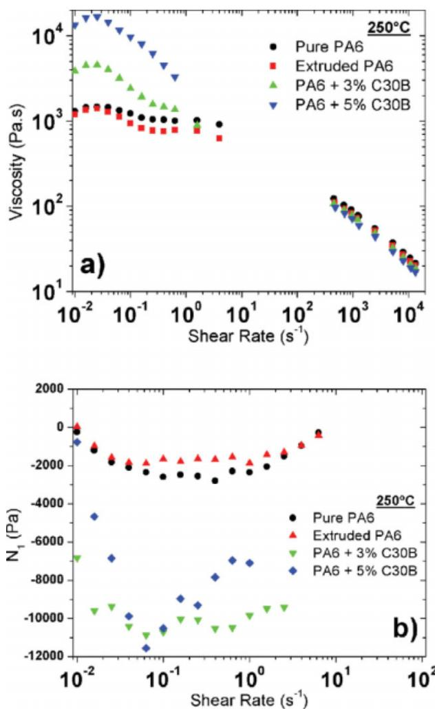
**Figure 6** Extruded PA6/MMT nanocomposites: (a) Shear viscosity and (b) First normal stress difference, both at 250°C. [Color figure can be viewed in the online issue, which is available at [www.interscience.wiley.com](http://www.interscience.wiley.com).]
