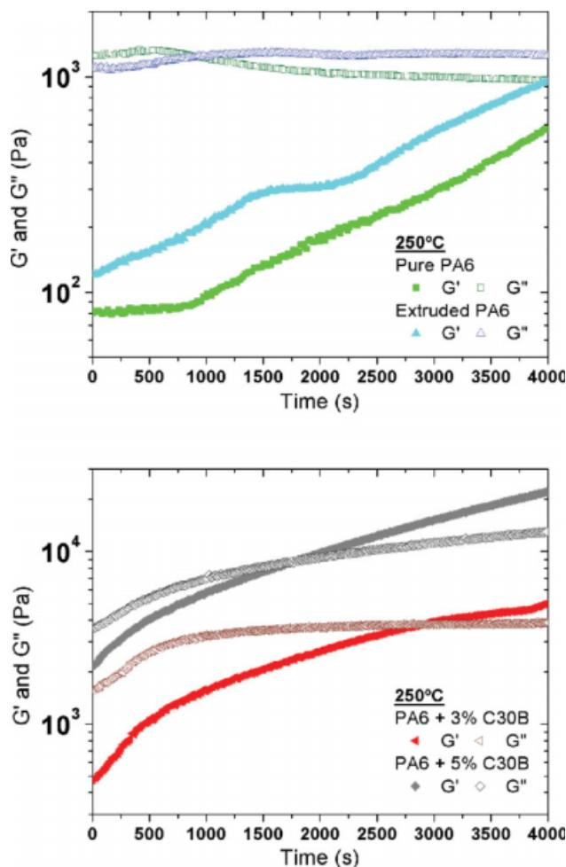
**Figure 8** Storage and loss modules of the nanocomposites as a function of time (250°C). [Color figure can be viewed in the online issue, which is available at [www.interscience.wiley.com](http://www.interscience.wiley.com).]
