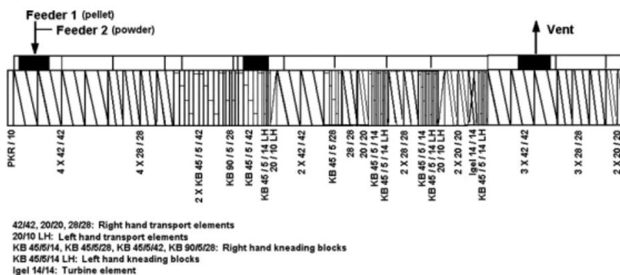
**Figure 2** Profile of the twin screw extruder used in this work.<sup>13</sup>
