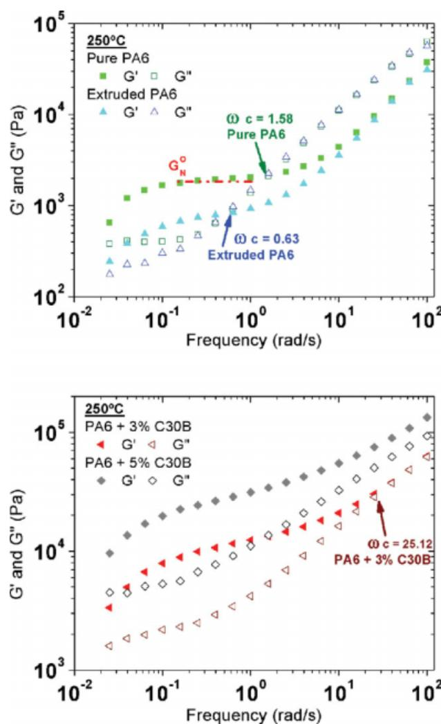
**Figure 7** Dynamic rheological properties of the extruded nanocomposites, at 250°C. [Color figure can be viewed in the online issue, which is available at [www.interscience.wiley.com](http://www.interscience.wiley.com).]
