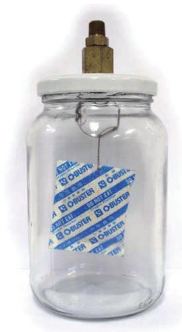
Figure 1. Hermetic absorption cell with a saturated salt solution for relative humidity control.
