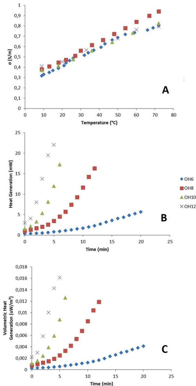
**Fig. 3.** Operating parameters for OH processing of flavored milk from 9 to 72 °C. (A) electrical conductivity ( $\sigma$ ); (B) heat generation; (C) volumetric heat generation. OH6, OH8, OH10 and OH12: Ohmic heating at 5.22, 6.96, 8.70 and 10.43 V/cm, respectively.
