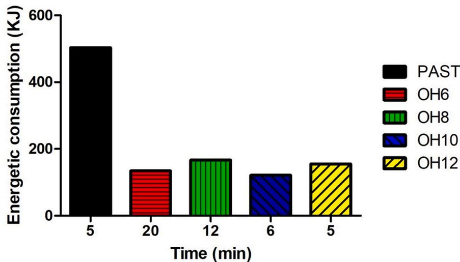
Fig. 4. Comparison of energy consumption (KJ) between conventional heating (PAST) and ohmic heating. OH6, OH8, OH10 and OH12: Ohmic heating at 5.22, 6.96, 8.70 and 10.43 V/cm, respectively.
