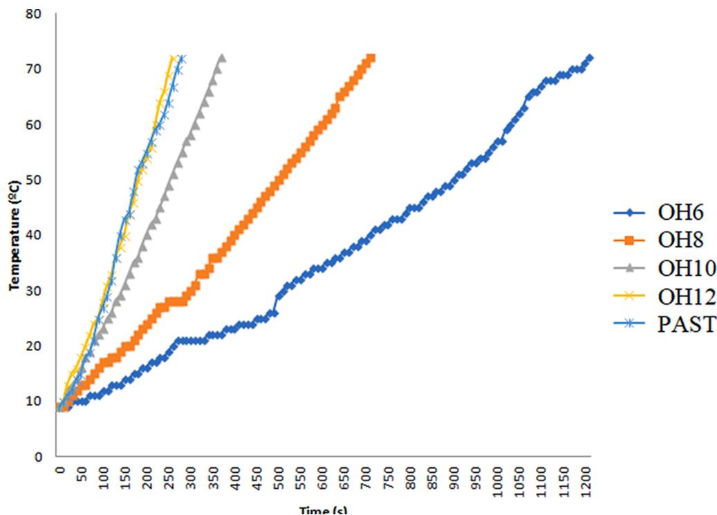
Fig. 2. Behavior of the time/temperature binomial of samples during ohmic heating processing and conventional treatment. OH6, OH8, OH10 and OH12: Ohmic heating at 5.22, 6.96, 8.70 and 10.43 V/cm, respectively. PAST: Conventional pasteurization.
