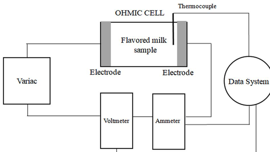
Fig. 1. Schematic diagram of ohmic heating system.
