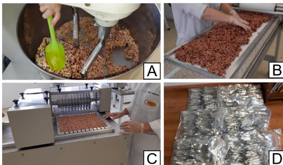
Fig. 1. Steps of fruit and cereal bar preparation. A) Homogenization, B) Laminating, C) Cut, and D) Storage. Source: Authors.
