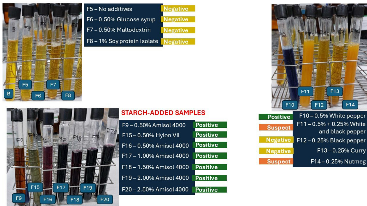
Figure 2. Visual appearance of test tubes after Lugol’s test compared with control tube “B”.
